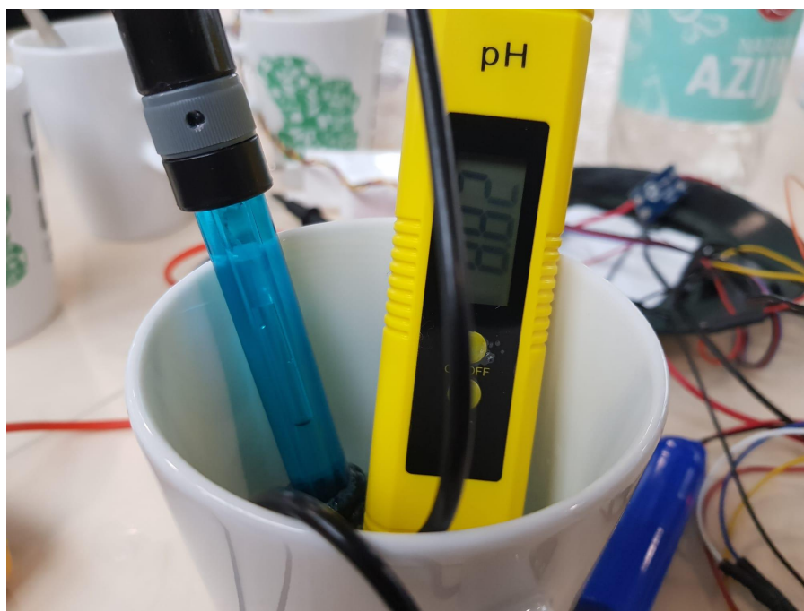
Figure 4. Validating sensor readings with a pH metre in tea
