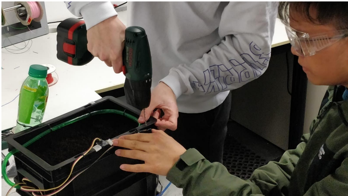
Drilling cable and tubing holes.
