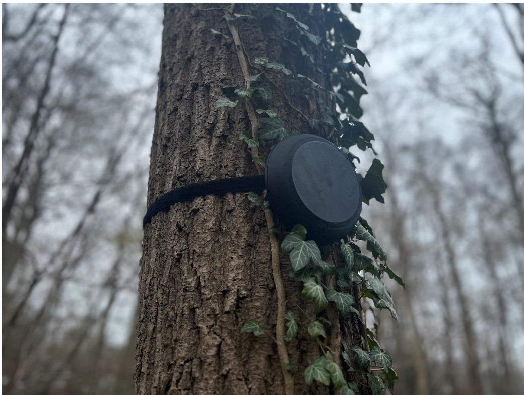
Appendix 4. Picture of the device placed in the wild. The prototypes were initially attached to objects with Velcro stripes.
