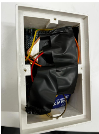
GPS Collar (Antenna, Arduino, Power Supply)
